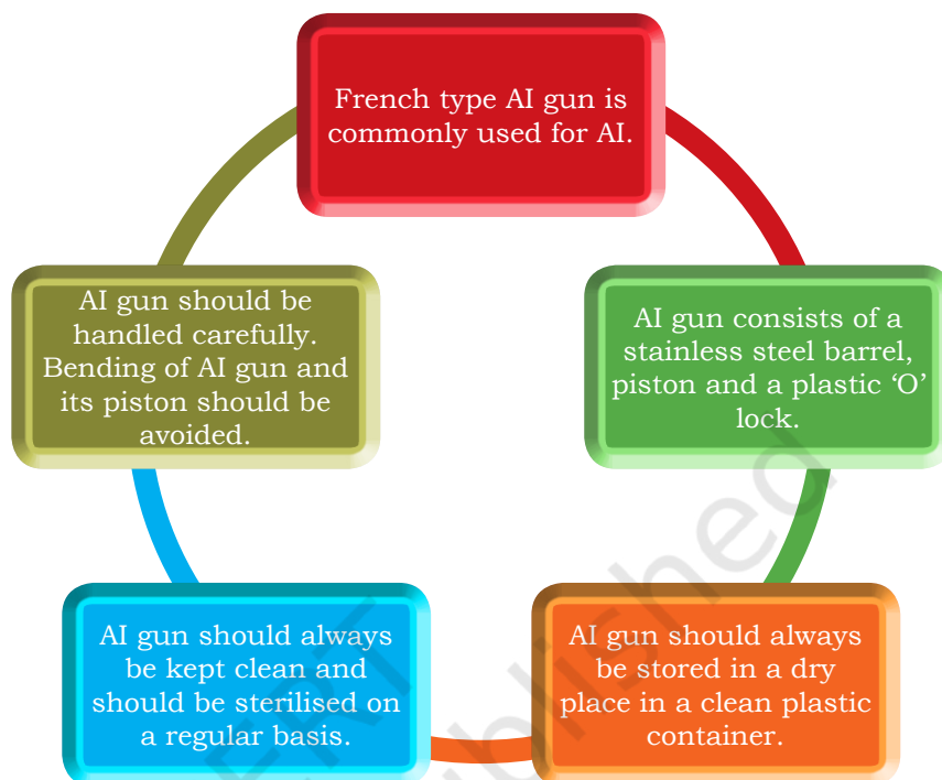
Fig. 4.45: Precautions to be taken while handling an AI gun
