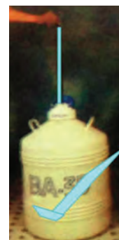
Fig. 4.42: Routinely check the level of \text{LN}_2 , preferably, twice in a week
